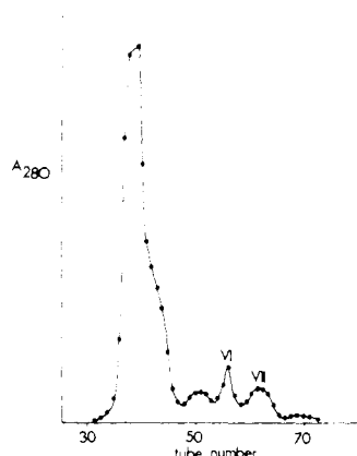
FIGURE 2: The elution profile of complex III eluted through Sephadex G-100 superfine in 6 M Gdn-HCl. The first peak eluting after the void volume was a polypeptide(s) of molecular weight 18 000. This is an impurity or possibly an aggregate of smaller subunits which is found in some preparations (see the text). Polypeptides VI and VII were separated. Polypeptide VIII was not detected off the column probably because of the low amount by weight in the complex.
